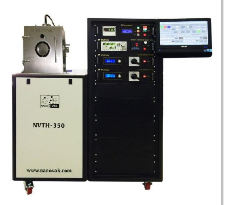
Box type Physical Vapor Deposition system is based on prismatic vacuum chamber. Multi-layered thin films of four different materials can be prepared by NVTH system. System can be tailored to fit user desires in order to produce multilayered, nanosize metallic, oxide, fluoride or nitride films, such as Si, Al, Ti, SiO, Au, Ag, WO, BaF<sub>2</sub>, MgF<sub>2</sub>. System can co-evaporate from any two sources.
